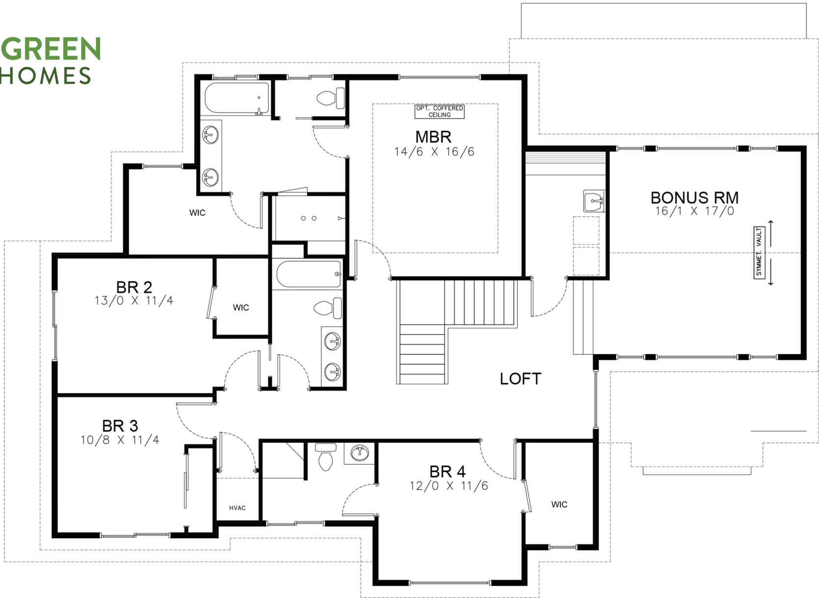
PLAN 3311 66'6" W x 43'9" D UPPER LEVEL, 1928 SF, 8' Ceiling Evergreen Homes NW Copyright 2016
